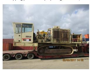
$2^{nd}$  shipping place – the mast: L 14,25m x W 1,7m x H 2,2m, Weight – 13 tons. Looks like:
